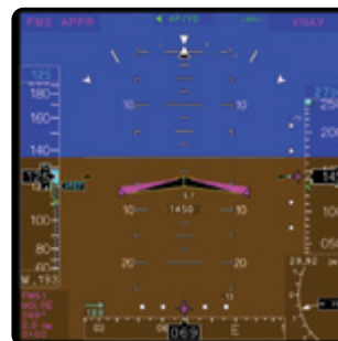
Full Primary Flight Display Mode with V-Bar Overlay
