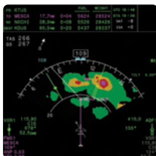
Nav Display with 120° Map View and Radar
