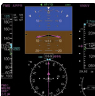
Composite Primary Flight Display with 360° HSI
