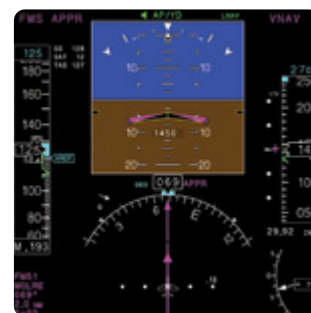
Composite Primary Flight Display with 120° HSI
