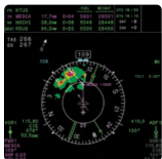
Nav Display with 360° Map View and Radar
